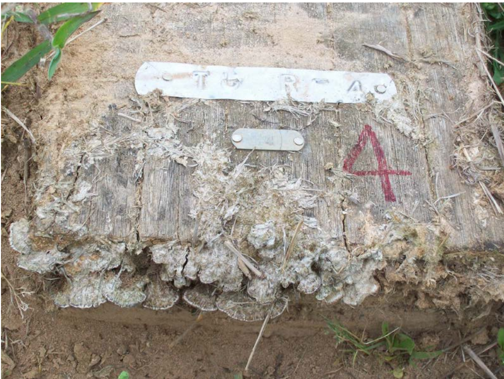
Figure 6 - Tie #4 with decay and fruiting bodies.
